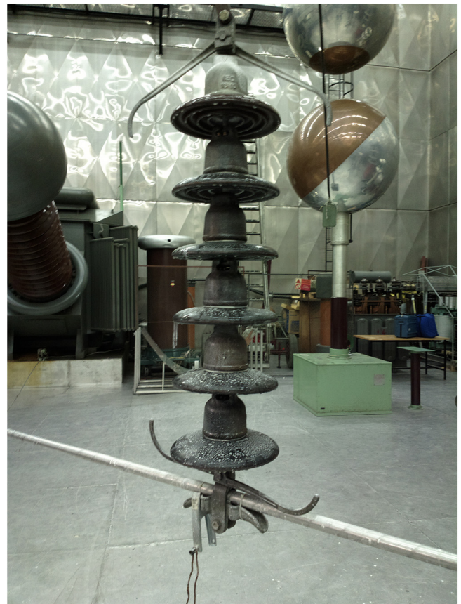
Fig. 1. Polluted test insulator.
